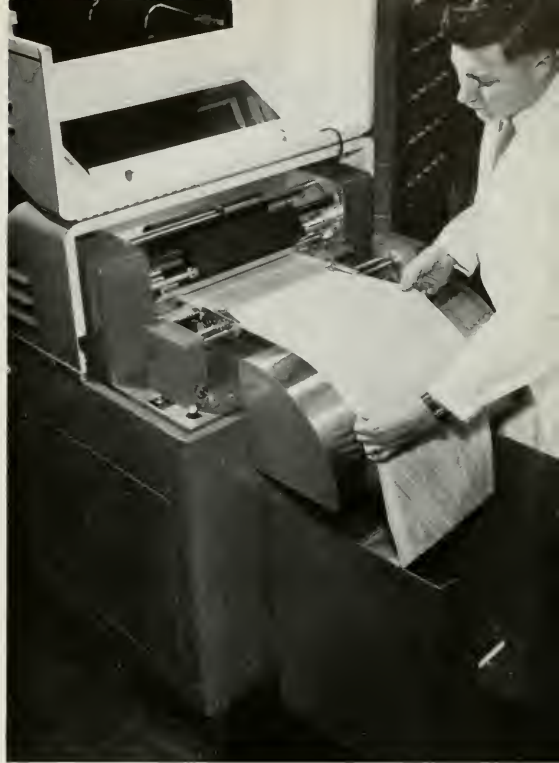
BIZMAC's electromechanical printer, shown here, can turn out finished paperwork at 600 lines a minute.
